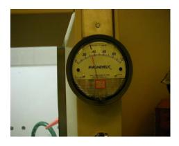
\*"Magnihelic gauge" – note normal gauge position. Significant deviation may indicate condition of low air flow.
