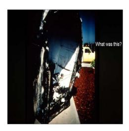
This picture shows a UCI lab refrigerator which exploded when chemicals were inappropriately stored in a unit which was not designed for flammables storage.
