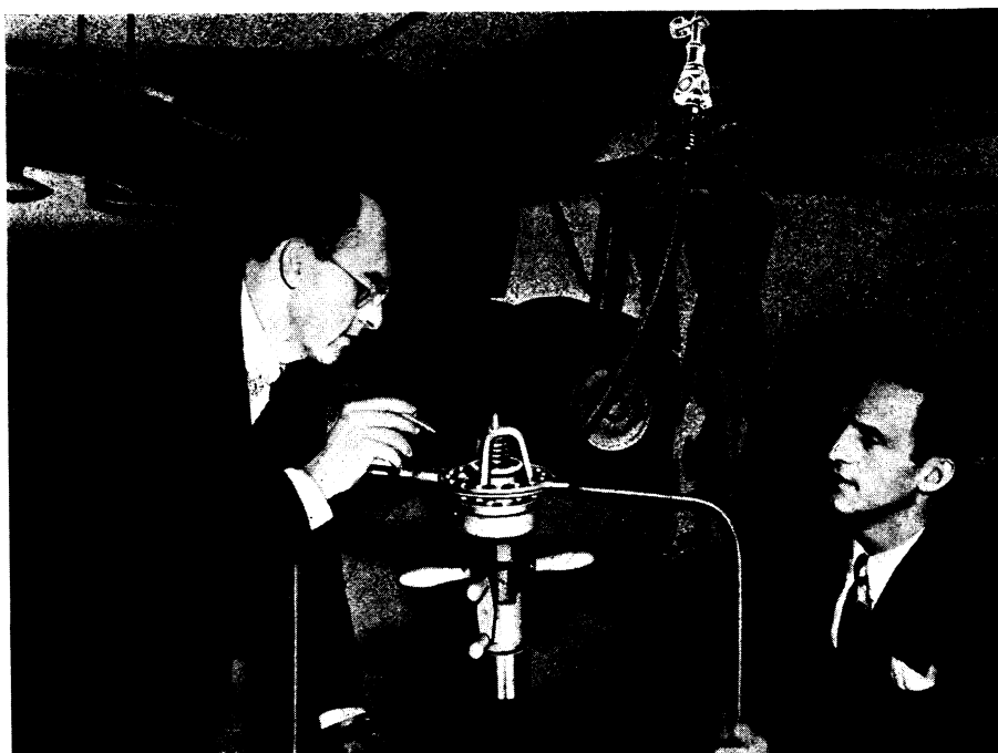
REFUELING VALVE —Underwing valve cuts down refueling delays.
