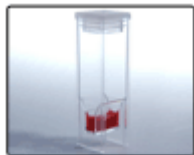
Small volume polystyrene cuvette with lid.
